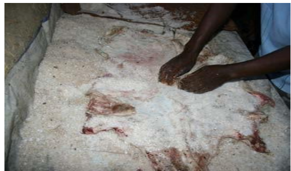
Figure 5. Salting skins on a cement floor. Figure 6. Salting practice ESGPIP.
